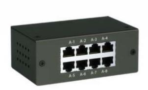
Allows to increase the number of sensors connected to any monitoring unit. Adds 8 analog sensors. Connects on CAN port and allows further CAN daysy chain connection. Sensors connected to the extension unit appears in the system automatically. Max. distance from the monitoring unit is 225 meters
